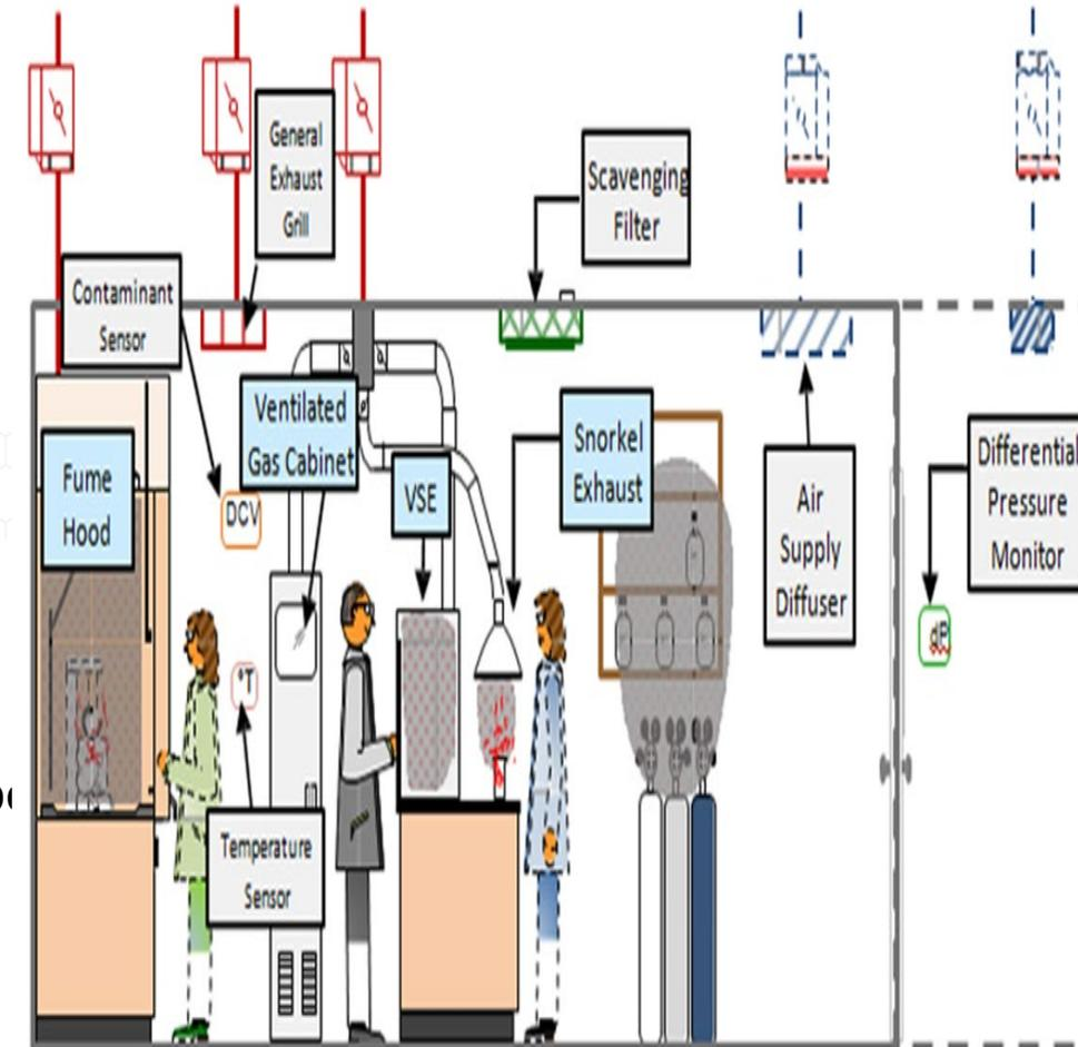
Figure 1 Side view of lab depicting various ECDs and Lab Ventilation Components
